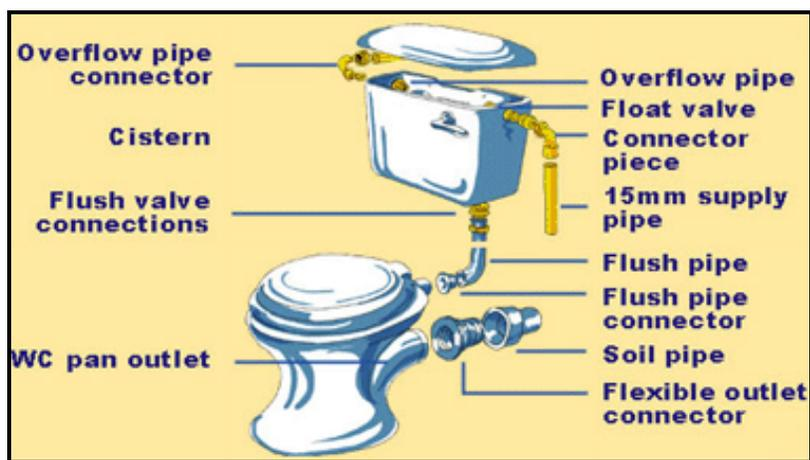
**Figure 5.1: Schematic Layout of Gravity Flush Toilet** (Courtesy [www.waterwise.co.za](http://www.waterwise.co.za))
