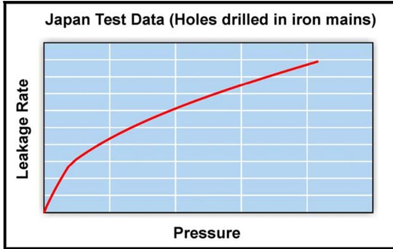
Figure 2.18: Theoretical Pressure / Leakage Relationship
