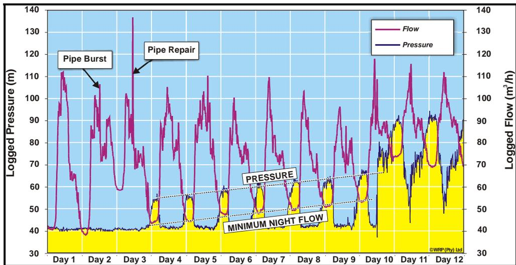
**Figure 3.4: Logging Results from Test Data used to Calculate N1 Value**
