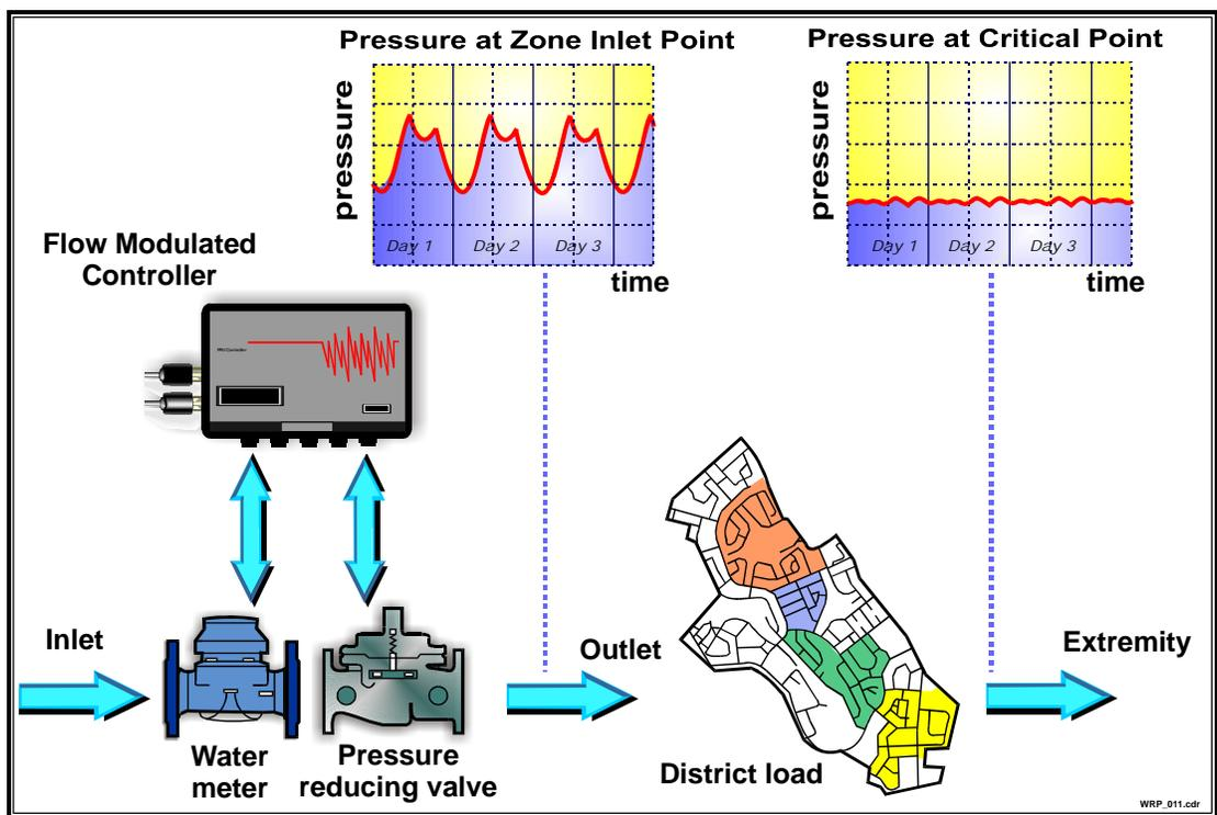
**Figure 4.9: Pressure Control using a Flow-Modulated PRV Controller**
