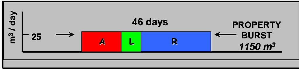
**Figure 2.11: Typical Duration and Losses from a Property Burst**
