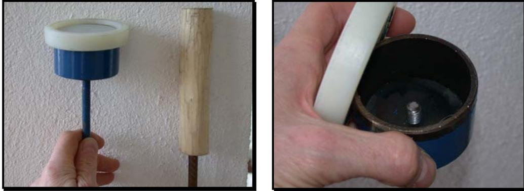
**Figure 2.8: Examples of commercial and “home made” sounding rods**
