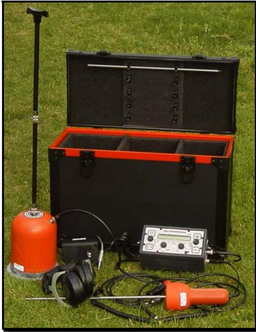
**Figure 4.20: Ground Microphone** (Courtesy Radiodetection (Pty) SA)
