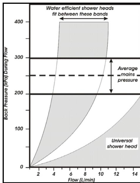
**Figure 5.14: Typical Flow Rate- Pressure Relationship for a universal showerhead and a range of water efficient showerheads (Adapted from Beith and Horton 1989)**
