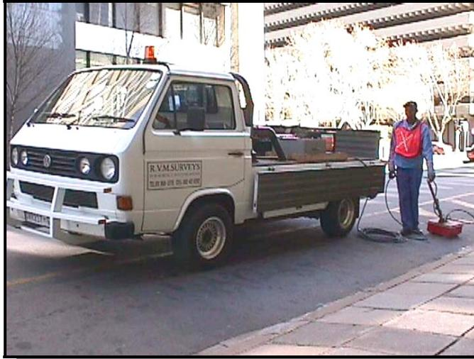
**Figure 4.24: Ground Penetrating Radar** (Courtesy RVM Surveys)
