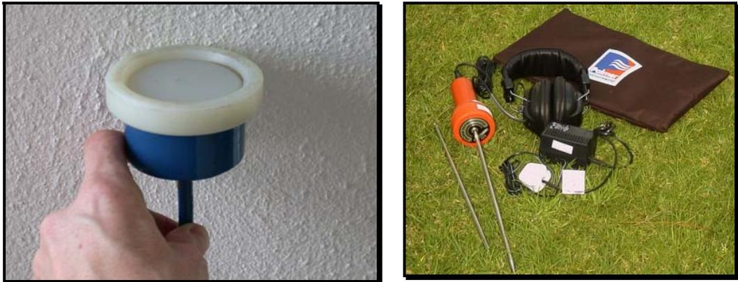
**Figure 4.19: Manual and Electronic Listening Sticks** (Courtesy Radiodetection (Pty) SA)
