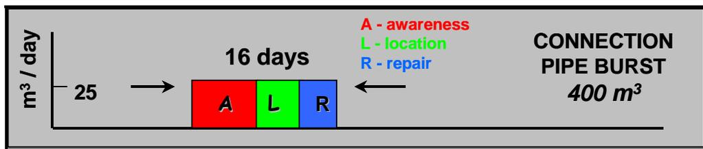
**Figure 2.10: Typical Duration and Losses from a Connection Burst**
