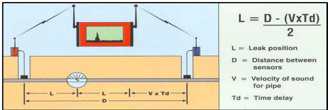
Figure 4.22: Theory of Leak Noise Correlation (Courtesy T Waldron, Wide Bay Water)
