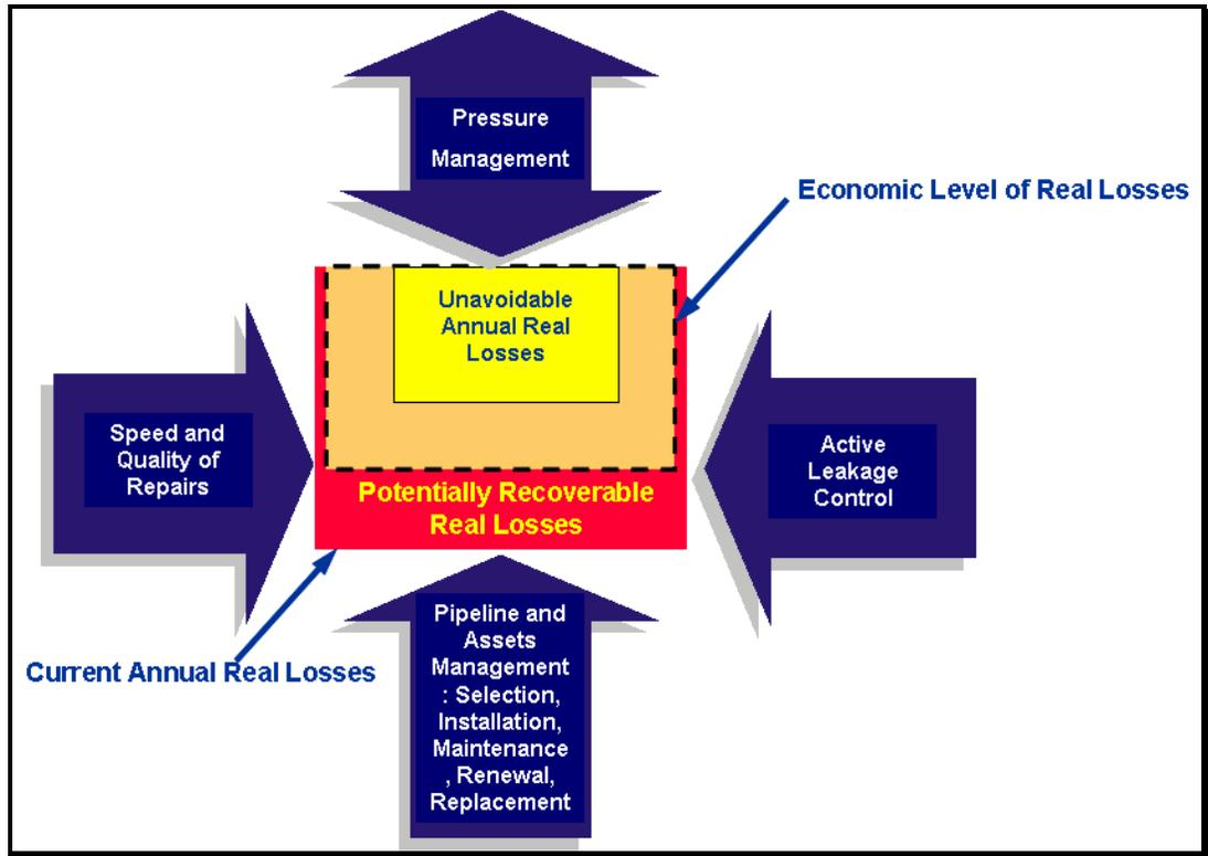
Figure 2.16: Influence on leakage of improving Active Leakage Control
