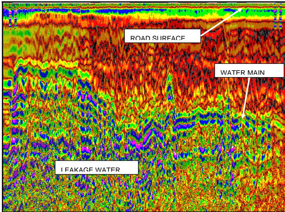
**Figure 4.25: Leakage Image created with GPR** (Courtesy RVM Surveys)
