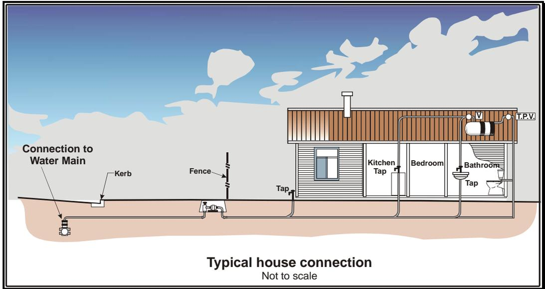
**Figure 2.6: Example of a House Connection to a Fully Serviced Property**
