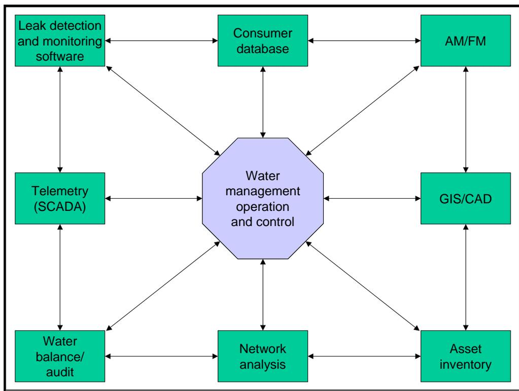
**Figure 3.1: Interaction Between Components of a Detailed MIS** (courtesy H Buckle)
