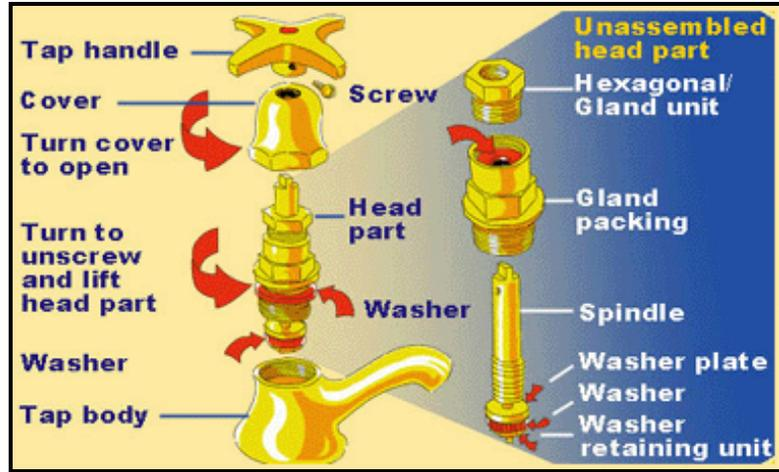
**Figure 5.13: Schematic illustration demonstrating how to repair a tap washer**
