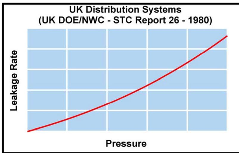
Figure 2.19: Leakage/Pressure Relationship in a Typical Water Supply System
