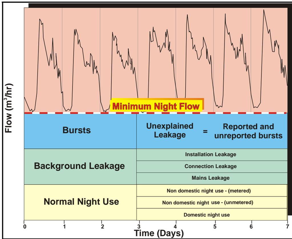
Figure 3.3: Components of Minimum Night Flow
