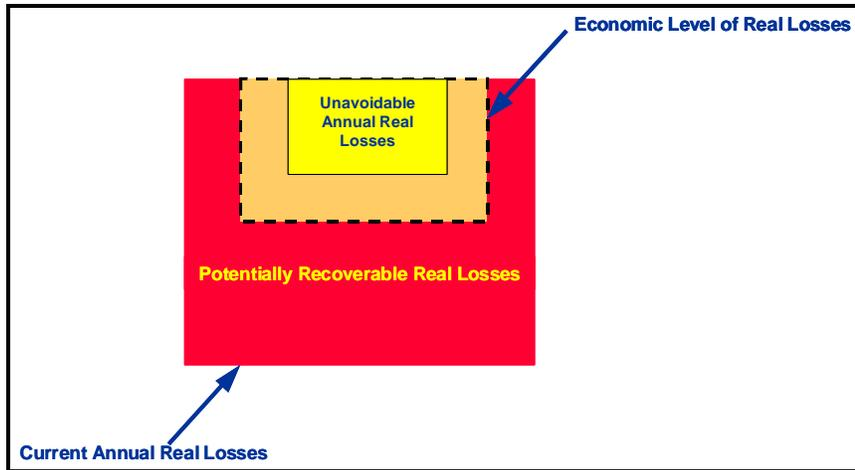
**Figure 2.12: Conceptual Representation of System Leakage**
