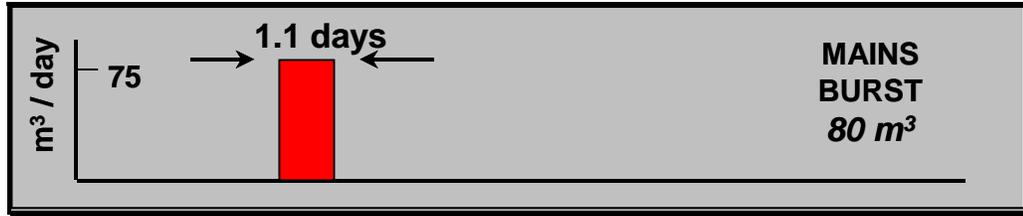
**Figure 2.9: Typical Duration and Losses from a Mains Burst**
