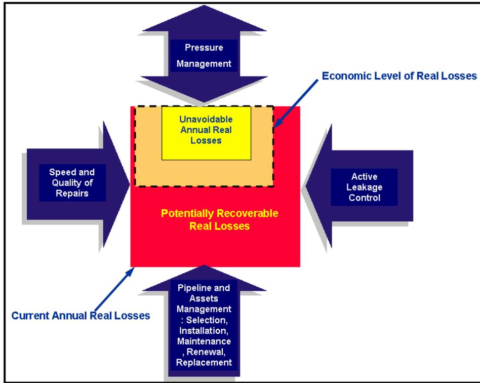
**Figure 2.14: Influence on Leakage of Improving Speed and Quality of Repairs**
