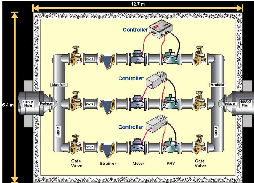
Figure F2: Schematic Layout of the 1065 mm diameter Installation
