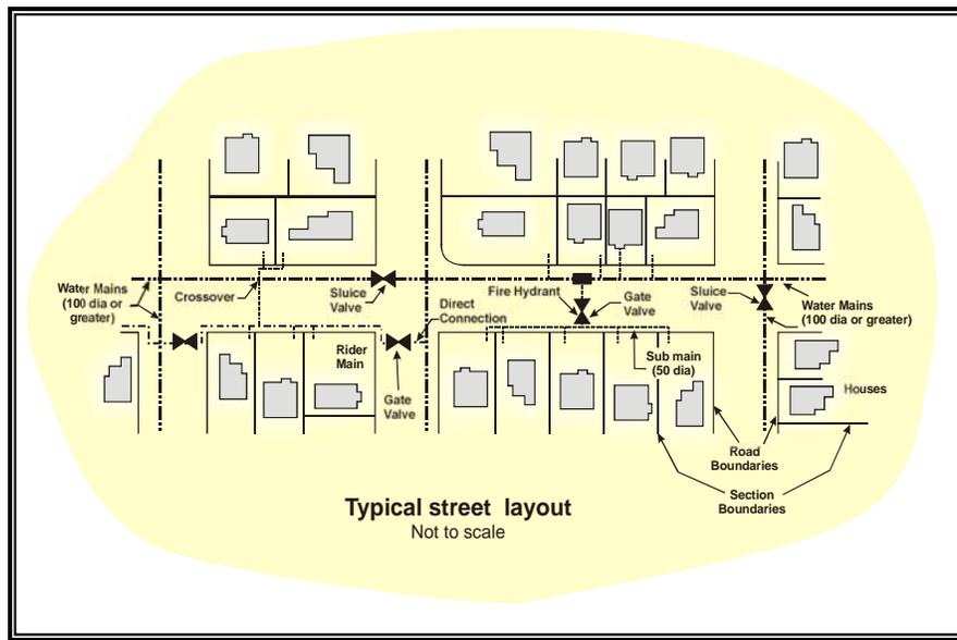
**Figure 2.5: Typical Water Distribution System**
