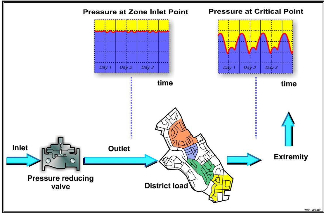
Figure 4.4: Pressure Control using Conventional Fixed Outlet PRV Controller
