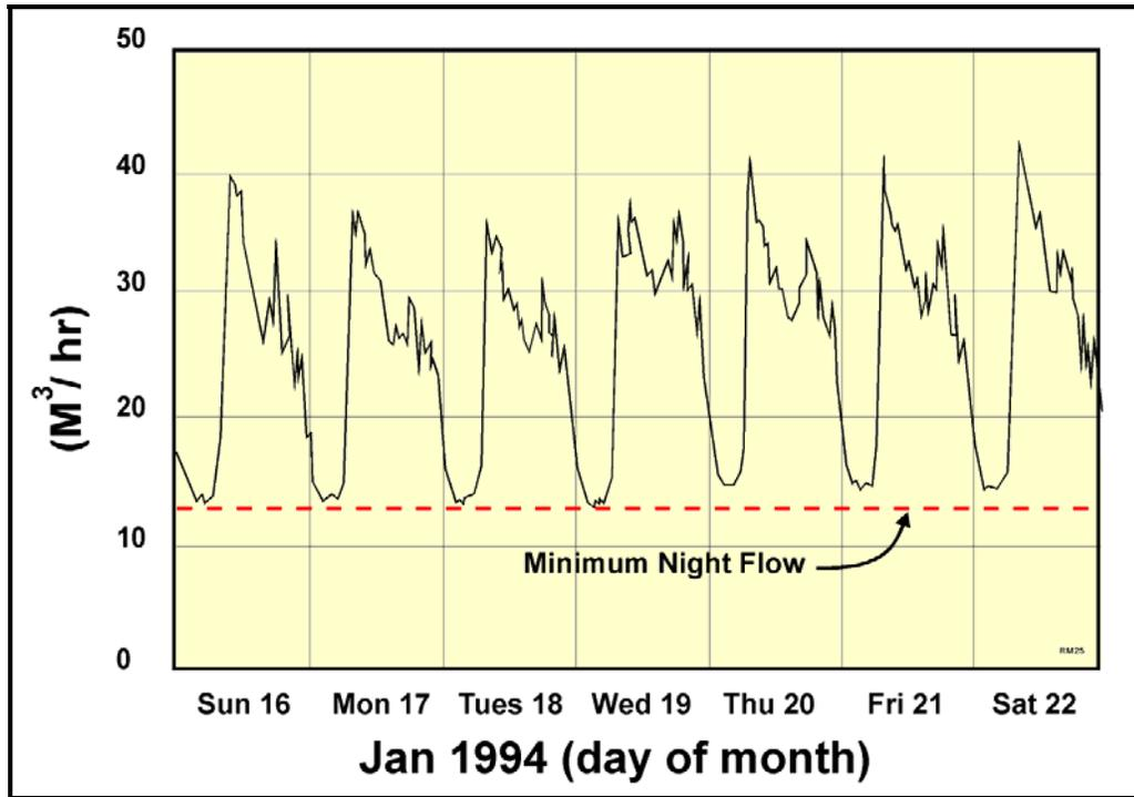
**Figure 3.2: Example of Flow Entering a Zone Metered Area**
