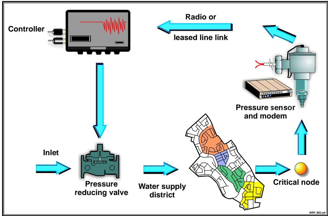
**Figure 4.10: Pressure Control using a Telemetry Linked Flow-Modulated PRV Controller**
