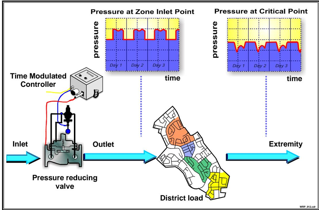
**Figure 4.7: Pressure Control using a Time-Modulated PRV Controller**
