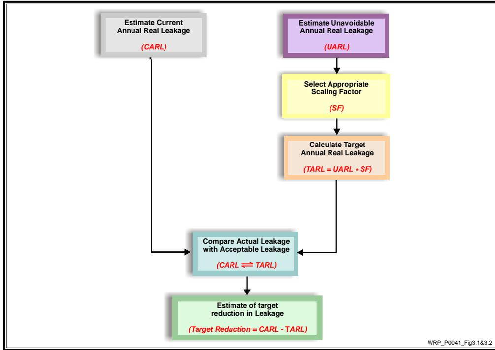
Figure 2.21: Procedure for Using BENCHLEAK
