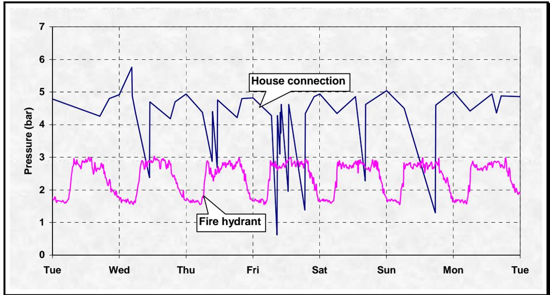
**Figure 4.12: Typical Pressure Loggings from a Fire Hydrant and House Connection**
