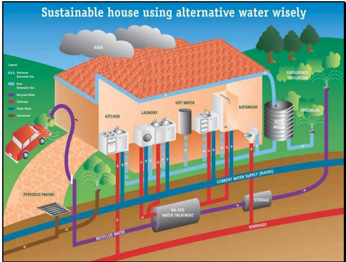
**Figure 5.17: Possible configuration for Grey Water Use in a household.**
