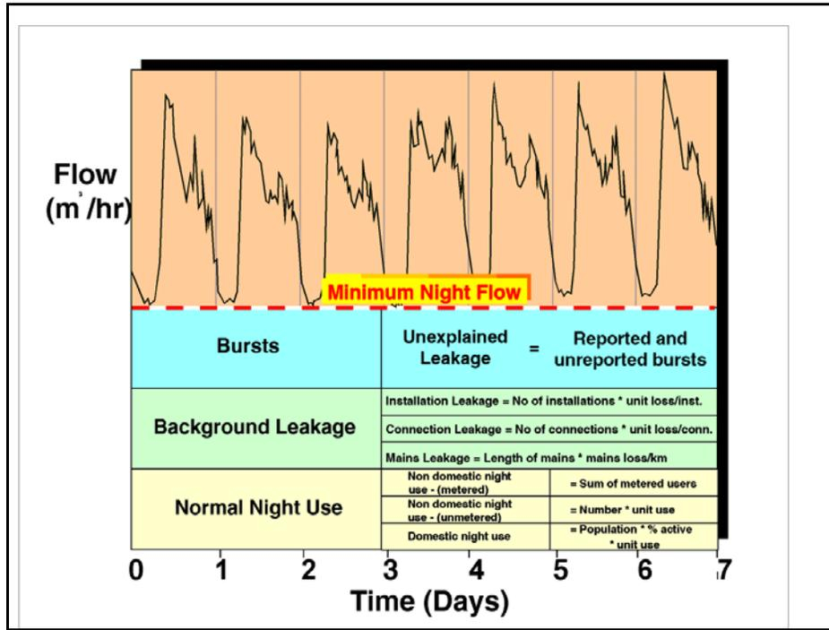
Figure E2: Components making up the minimum night-flow
